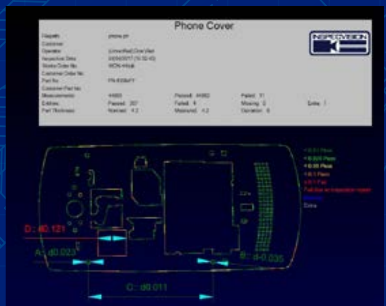
Figure 3: 2D Inspection with Deviation Map
